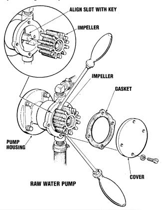
**CAUTION:** If any of the vanes have broken off the impeller they must be found to prevent blockage in the cooling circuit. They often can be found in the heat exchanger.
