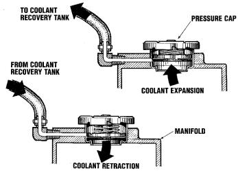
**NOTE:** Periodically check the condition of the manifold pressure cap. Ensure that the upper and lower rubber seals are in good condition and check that the vacuum valve opens and closes tightly. Carry a spare cap.
