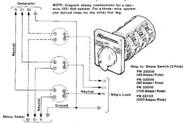
If the installer connects shore power to the vessel's AC circuit, this must be done by means of the Shore Power Transfer Switch. Set the transfer switch shown in the diagrams to the OFF position. This switch prevents simultaneous connection of shore power to generator output.
