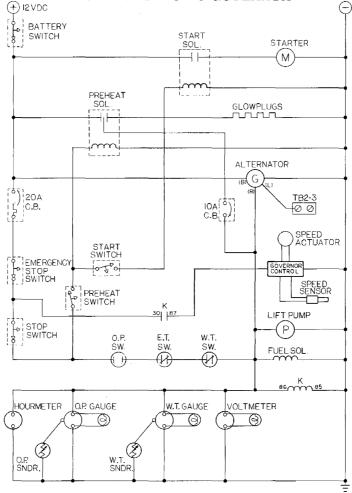
**NOTE:** An on-off switch should be installed in this circuit to disconnect the starter from the battery in an emergency and when leaving the boat. Twelve volt diesel engine starters typically draw 200 to 300 amps when cranking. A switch with a continuous rating of 175 amps at 12 VDC will normally serve this function, but a switch must never be used to "make" the starter circuit.
