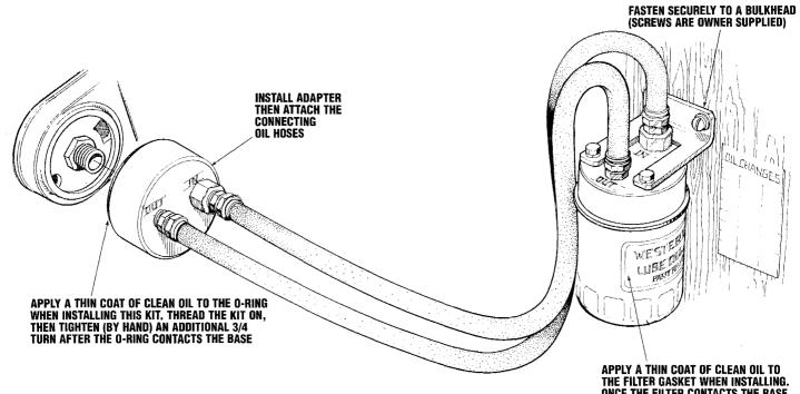
THE FILTER GASKET WHEN INSTALLING. ONCE THE FILTER CONTACTS THE BASE, TIGHTEN IT (BY HAND) A 3/4 TURN MORE.
