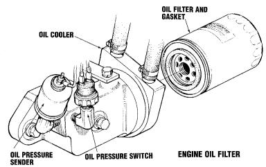
**NOTE:** Generic filters are not recommended, as the material standards or diameters of important items on generic parts might be entirely different from genuine parts. Immediately after an oil filter change and oil fill, run the engine to make sure the oil pressure is normal and that there are no oil leaks around the new oil filter.
