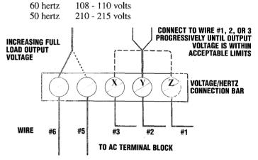
Should the voltage drop below the proper rate, loaded excitation can be increased to raise this voltage by repositioning connections on the Voltage/Hertz Connection Bar. Repositioning the two leads (red&white and yellow &white) from (Z) to (Y) or (X) will increase the loaded voltage out progressively in that order.
