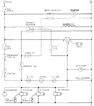
**NOTE:** An on-off switch should be installed in this circuit to disconnect the starter from the battery in an emergency and when leaving the boat. Twelve volt diesel engine starters typically draw 200 to 300 amps when cranking. A switch with a continuous rating of 175 amps at 12 VDC will normally serve this function, but a switch must never be used to "make" the starter circuit.
